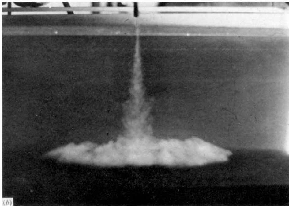
FIGURE 1. Plume of dyed fluid ( a ) immediately after striking interface and ( b ) 2 s later. Plume flux is 1 ml/s of salt solution, specific gravity 1.12. Heavier layer is salt solution, specific gravity 1.084, dyed blue. Froude number = 0.55.
